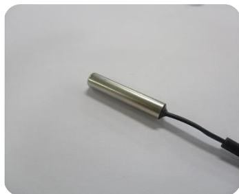
Thermistor Epoxy potting type Nickel plated Copper Alloy Case -30 to +120°C
