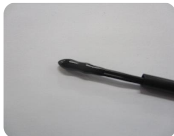
Thermistor Epoxy dipping type -30 to +80°C
